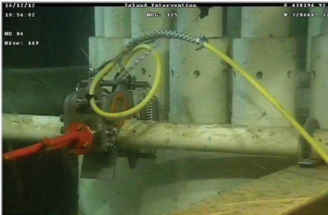
Figure 3 – Accelerometer attached to a subsea piping system.
