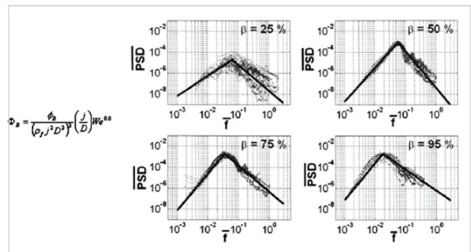
Figure 1 – Empirically derived forcing spectra for multiphase flow.
