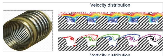
Figure 2 – Vorticity generation due to flow across a corrugated liner.
