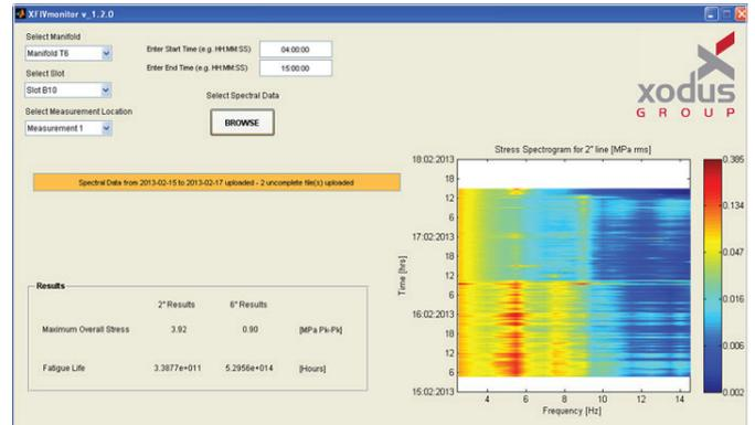
Figure 6 – Analysis of measured data.
