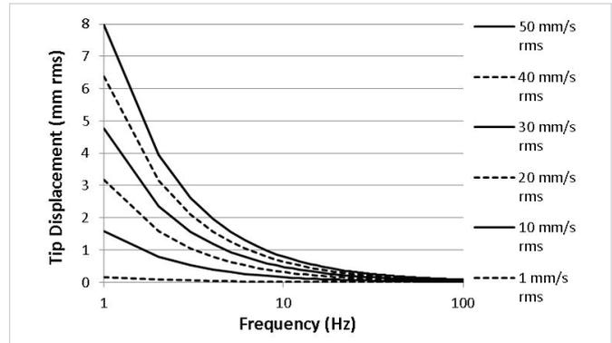
Fig. 2 – Displacement (mm rms) at tip (free end) of an SBC as a function of vibration magnitude (velocity) and response frequency.
