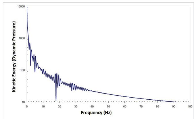
Fig. 3 – Turbulent energy distribution between 0 Hz and 100 Hz [1].
