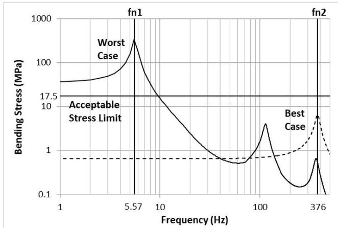
Fig. 6 – Peak bending stress of two different geometries.
