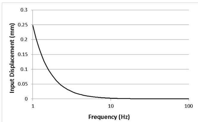
Fig. 5 – Input displacement as a function of frequency for a constant acceleration input.
