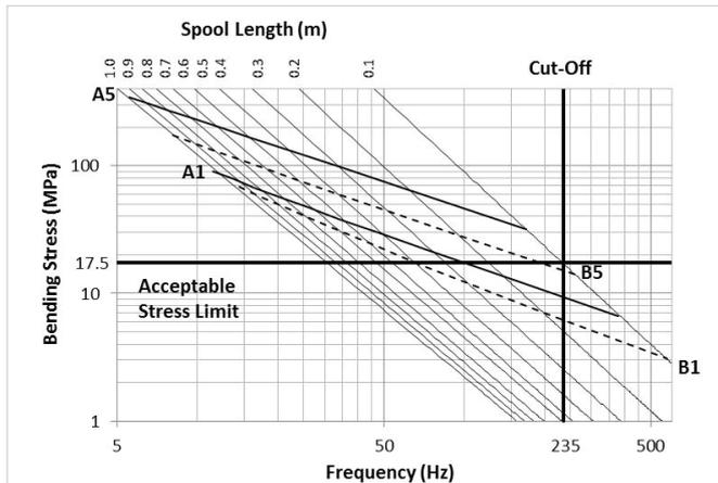
Fig. 7 – Bending stress for multiple geometries.
