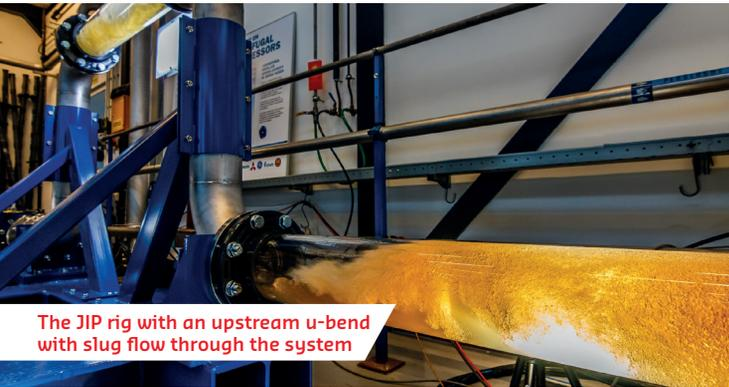
The JIP rig with an upstream u-bend with slug flow through the system
